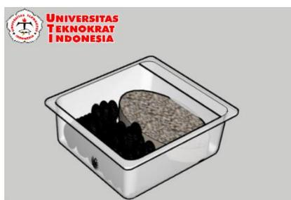
Gambar 2. Biofilter media bio rings dan bioball
