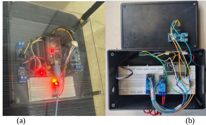
Gambar 4. Hasil rancangan (a) monitoring genset (b) monitoring rooftop
