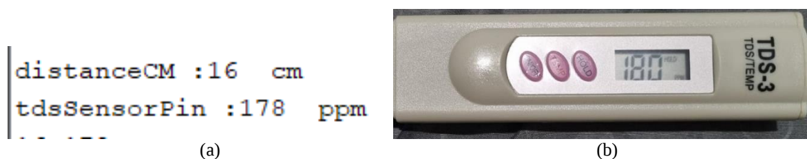
Gambar 5. Pengujian sensor TDS Meter (a) Serial monitor (b) TDS-3
